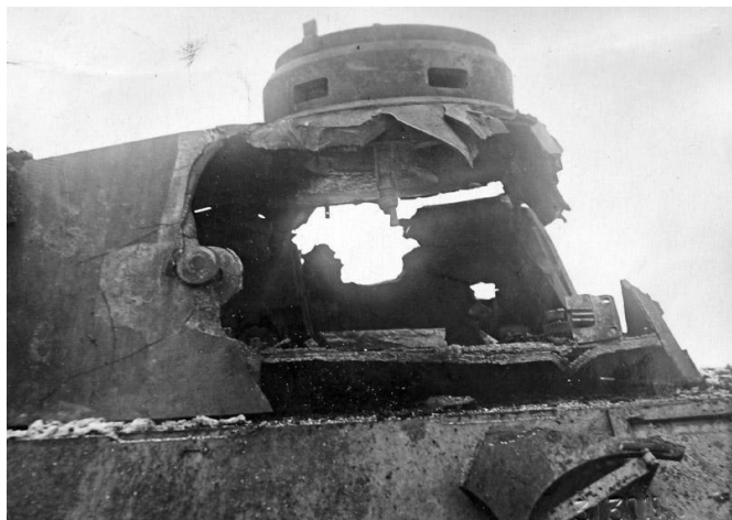
Effects of a 152mm hit against the 45mm, 25° sloped armor plate of a turret.
